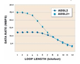
ADSL2+ can also be used to reduce crosstalk. ADSL2+ provides the capability to use only tones between 1.1 MHz and 2.2 MHz by masking the downstream frequencies below 1.1 MHz. This can be particularly useful when ADSL services from both the central office (CO) and a remote terminal (RT) are present in the same binder as they approach customers' homes. The crosstalk from the ADSL services from the RT onto the lines from the CO can significantly impair data rates on the line from the CO.
